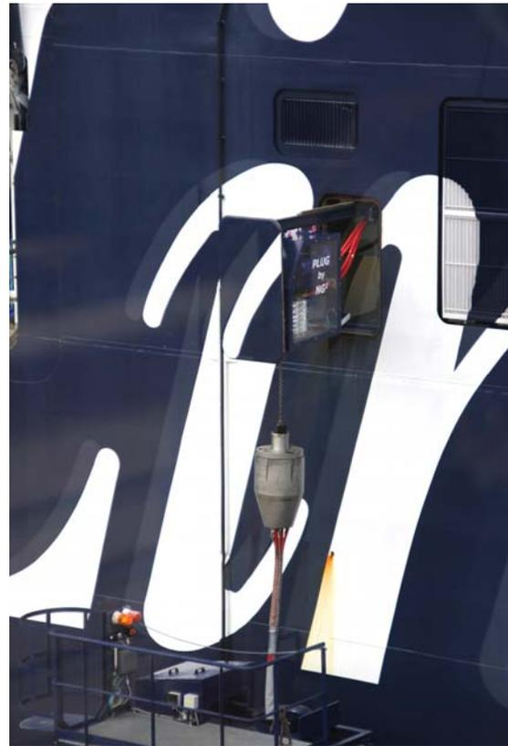
*No regular electrical outlet. Electrical connection to the ship is fully automated.*
